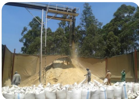
Picture 4: Coffee husk during the de-hulling process in Kofinaf.
